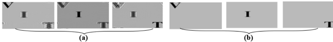
Fig. 2: Reconstructed intensity images using deep learning U-network at different depth planes (a) without image segmentation and (b) with image segmentation
