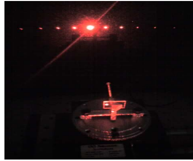
Fig. 8: Different order of phase grating at wavelength 633 nm (vertical polarisation)
