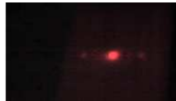
Fig. 10: Order of phase grating at wavelength 1550nm (horizontal polarisation)
