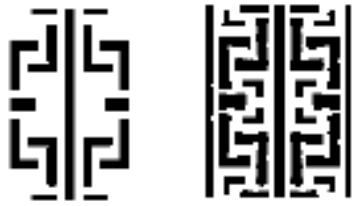
Figure 8. (a) Input layout (b) Modified layout using inverse lithography technique
