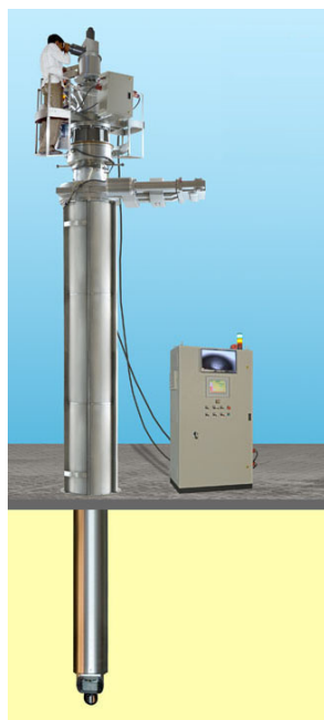
Fig.1 Photograph of periscope cover gas, which is 150° C and radiation field of 1.3 R/hr. Additional accessories such as Leak Tight Chamber, Preheating Chamber and Gate Valves ensure periscope introduction and inspection in a leak tight manner. The Periscope is also sealed, purged with Argon and maintained at slightly higher pressure than the reactor cover gas, ensuring no leakage of reactor argon in case of seal failure. The complete assembly consisting of viewing and illuminating
