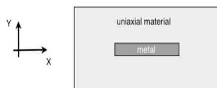
Figure 1: Geometry of the waveguide structure: a metal strip embedded in a uniaxial material.
