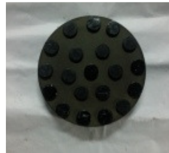
Fig2:- (c) Pitch buttons on cast Iron tool
