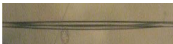
Fig 2: Fabricated etched fiber optic coupler
