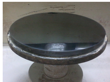
Fig1:- Si window blocked on a cast iron tool with the help of pitch
