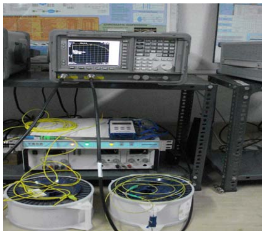
Figure2.Experimental setup for 900MHz RF signals transmission through fiber.
