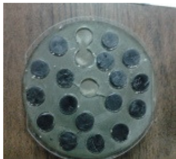
Fig2:- (b) pitch button with glass plate
