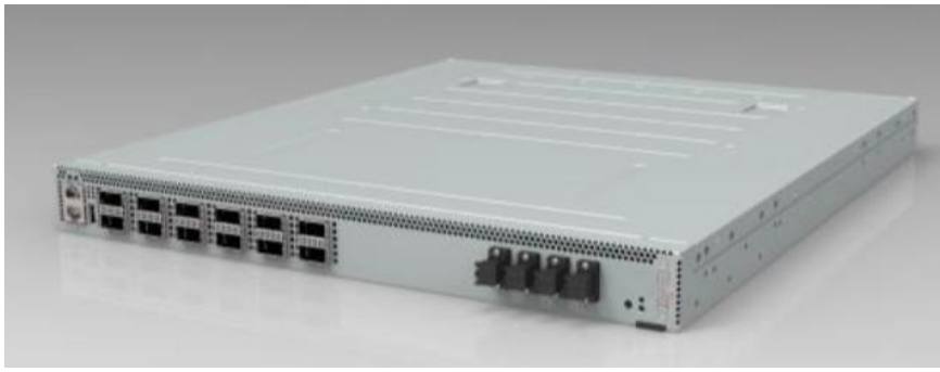
Voyager transponder with 12 QSFP28 ports and 4 x200G DWDM line ports
